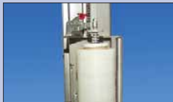
Mandrel with Ergonomic Handle Design Retains the Tension After the Film Roll is Replaced
