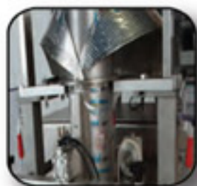
Quick Disconnect Former for easy cleaning and maintenance
