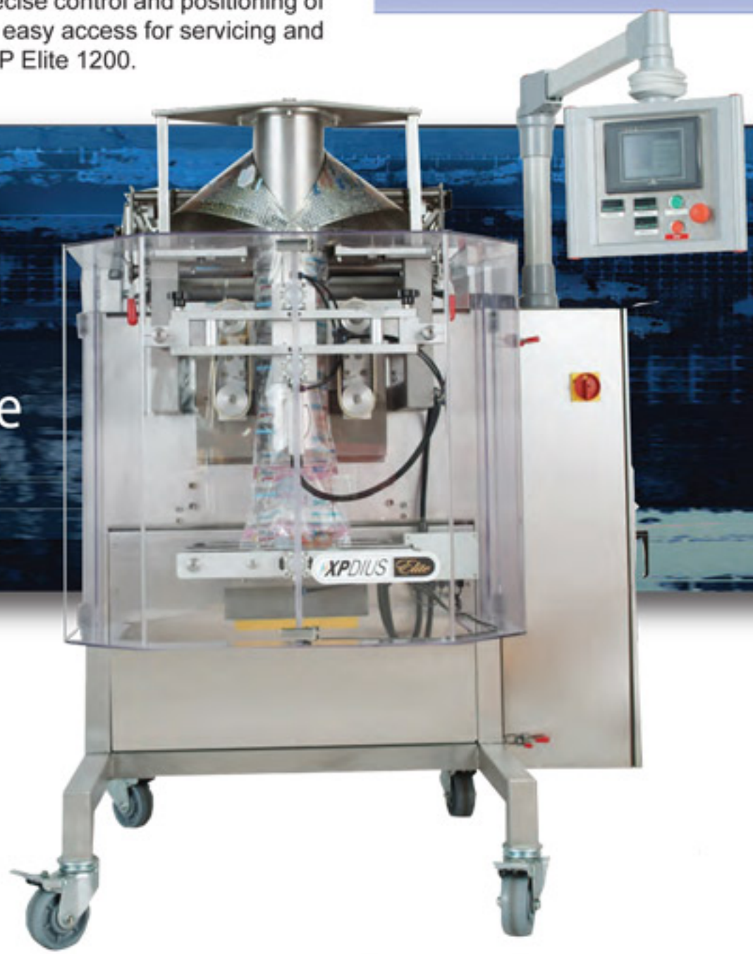
Quick Disconnect Former for easy cleaning and maintenance
