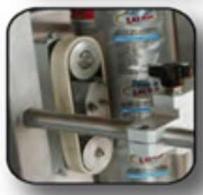
Servo-Driven Pull Belts smooth operation and precision
