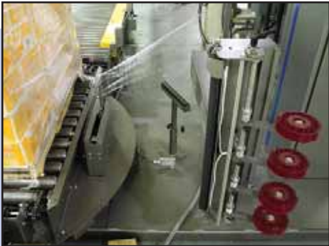
Film Clamp/Cut/Wipe Assembly Cuts and Attaches the Film Tail to the Pallet Load
