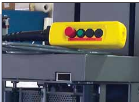
Remote Pendant with Emergency Stop, Cycle Start and Stop
